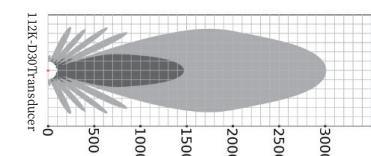
Dark color: 75mm diameter PVC pipe Unit: mm
